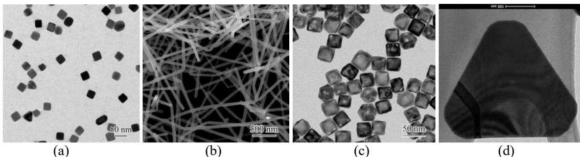
**Fig. 2: Different shapes of nanoparticles prepared for the study (a) nanocube (b) nanowire (c) nanocage (d) nanoplate*****Optimized the concentration of nanoparticles to be sprayed***
