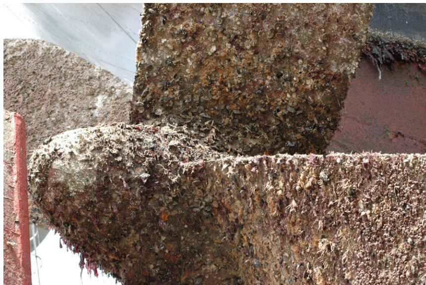
Messy business: Biofouling on the hulls (and even propellers) of ships is a major economic problem. (Photo: Gail Ashton, Smithsonian Environmental Research Center.)
